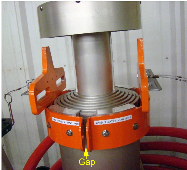
Both Clamps and Vertical Support on Mast
