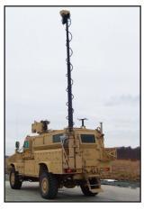
The CCTV mast is a Rapid deployment and retraction elevation system with On-The Move capabilities when extended that allow surveillance missions to remain covert and safe.
