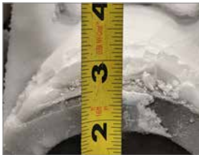
The Night Scan Powerlite IQ was tested at -15° F (-26° C) with a ¼" (6mm) of ice
