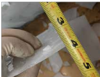
The Night Scan Powerlite IQ was tested at -15° F (-26° C) with a ¼" (6mm) of ice
