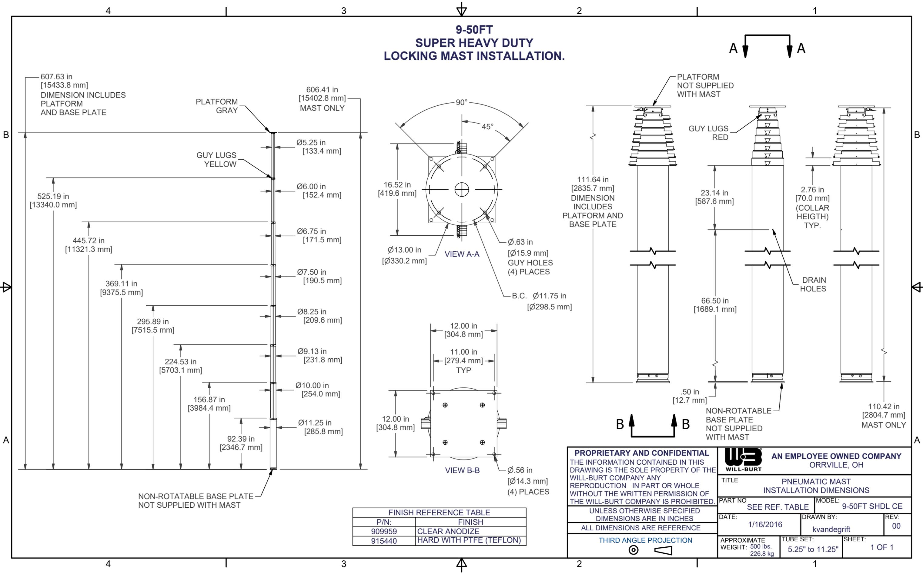
607.63 in [15433.8 mm] DIMENSION INCLUDES PLATFORM AND BASE PLATE
