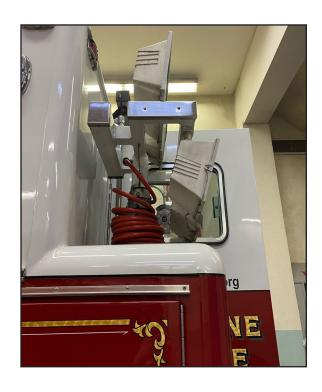
The evolution of the Night Scan has increased the number of options for height and payload capabilities, added different light fixtures to fit all spaces on a vehicle, along with the option to have a wireless remote controller to deploy a light tower while outside of the vehicle.
