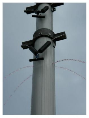
Figure 3-9 Water and Antifreeze Released out the Weep Holes
