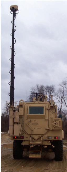
The Will-Burt Company has built upon pneumatic mast technology that has been refined over the past 30 years to provide a solution that meets all specifications for the REF Counter Sniper Program. This technology has helped keep our soldiers safe in Afghanistan and Iraq through the VOSS and VOSS II programs.
