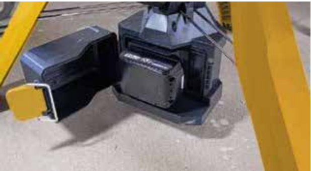
Protective IP54 Battery Housing
