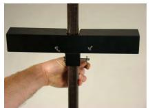
Figure 4-80 Use the Hitch Pin to Attach the Step to the Tripod
