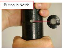
Figure 4-32 Place a Tube into the Bottom
