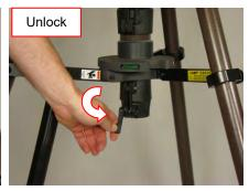
Figure 4-13 Lock the Upper Clamp and Unlock the Lower Clamp
