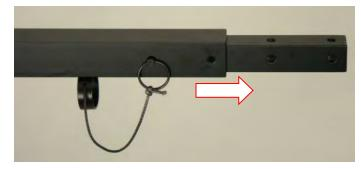
Figure 4-51 If Required, Extend and Pin
