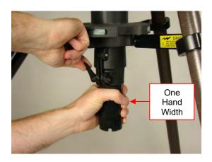
Figure 4-75 Lock Lower Clamp
