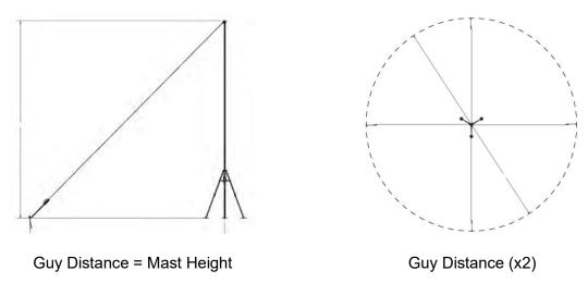
Figure 4-29 Drive the Stakes a Distance Equal to the Mast Height from the Center of the Mast
