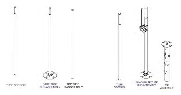
Figure 2-1 Telescoping Mast Parts (Not to Scale)
