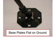
Figure 4-11 Open the Tripod
