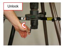
Figure 4-38 Lock the Upper Clamp and Unlock the Lower Clamp
