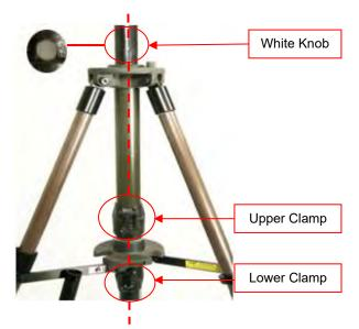
Figure 4-39 Insert Top Tube from the Top of the Tripod
