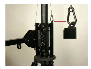
Figure 4-56 Connect to Eyelet
