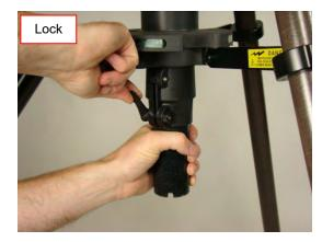
Figure 4-15 Lower Top Tube Until There is One Hand Width from the Bottom of the Tube and Lock the Lower Clamp
