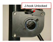
Figure 4-66 Unlock Winch Spool
