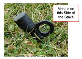
Figure 4-65 Drive Each Stake into the Ground at a 45° Angle
