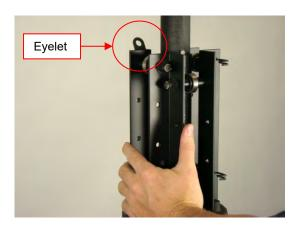
Figure 4-44 Ensure the Eyelet is on the Backside of the Mast
