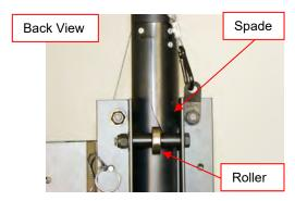
Figure 4-82 Turn the Winch Handle Counterclockwise to Raise the Payload
