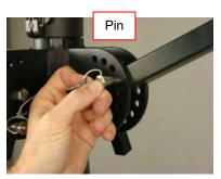
Figure 4-20 Pin Arm in Place
