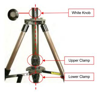
Figure 4-14 Insert Top Tube from the Top of the Tripod
