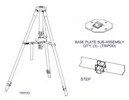
Figure 2-2 Tripod, Base Plate Assembly and Tripod Step
