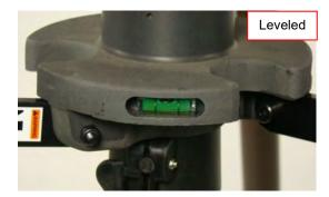
Figure 4-61 Adjust Legs as Needed and Consult Bubble Level to Ensure Tripod is Level
