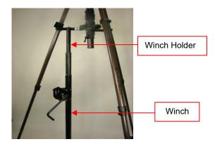
Figure 4-67 Use the Hitch Pin to Attach the Handle to the Winch
