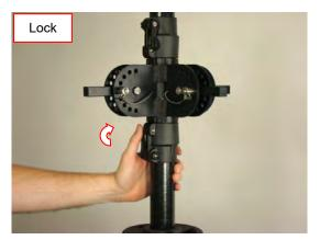
Figure 4-19 Lock Top and Bottom Clamps
