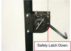
Figure 4-81 Unlock Winch Spool
