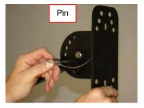
Figure 4-21 Pin Payload Adaptor in Place
