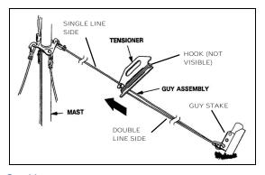
Figure 4-37 Tighten Guy Lines
