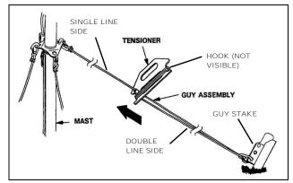
Figure 4-79 Tighten Guy Lines
