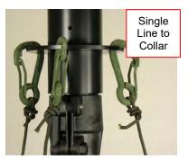
Figure 4-23 Connect Hook Ends to 4-Way Guy Collar
