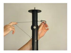
Figure 4-55 Feed Through Pulley
