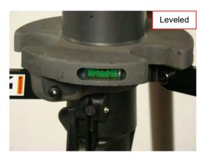
Figure 4-25 Adjust Legs as Needed and Consult Bubble Level to Ensure Tripod is Level
