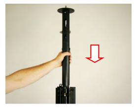
Figure 4-43 Insert Tip Tube
