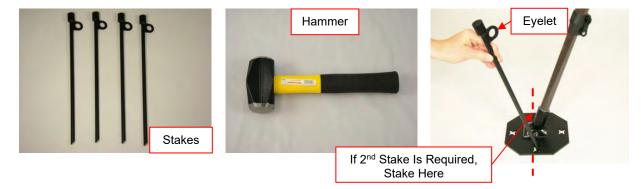
Figure 4-62 Stake the Tripod
