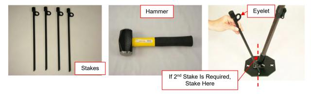
Figure 4-26 Stake the Tripod
