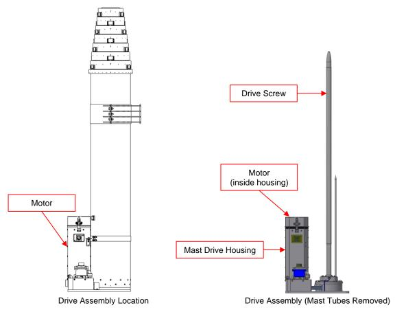
Figure 1-4 Drive Assembly (Not to Scale)
