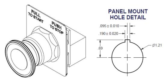
Figure 2-10 Emergency Stop Switch Kit
