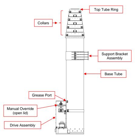
Figure 1-1 Mast (10-Meter Stiletto HD P/N: 711991091 Shown)
