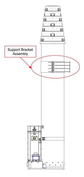
Figure 1-5 Support Bracket Assembly
