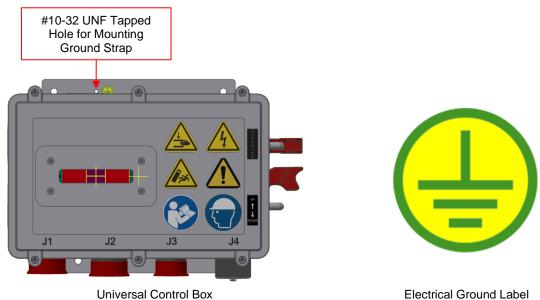
Figure 2-7 Universal Control Box Ground Location
