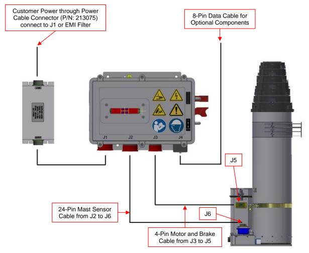
Figure 2-8 Stiletto HD Wiring (Not to Scale)
