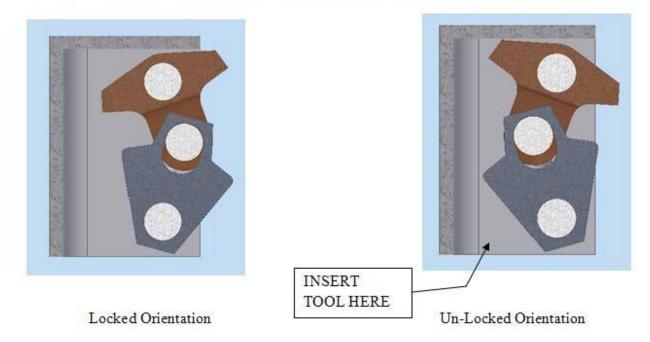
Figure 3-8 Lock Housing Ice Removal
