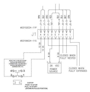
Figure 2-11 Power Cable Connector Wiring
