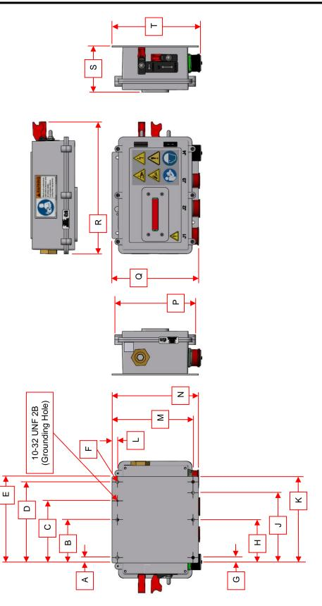
Figure 2-3 Universal Control Box Installation Dimensions (Measurements in Inches)
