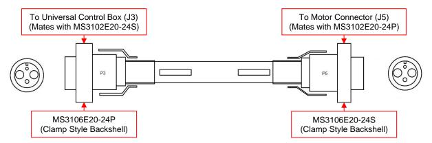
Figure 1-6 Motor and Brake Cable
