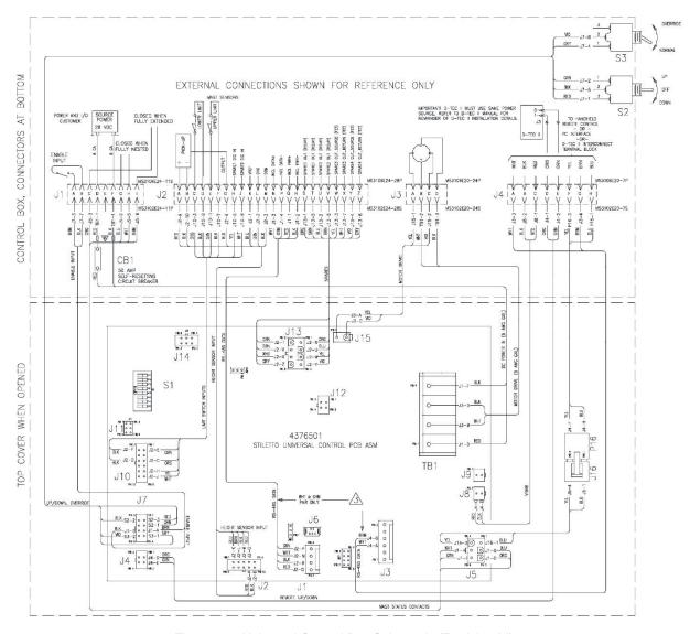
Figure 2-9 Universal Control Box Schematic (Revision M)
