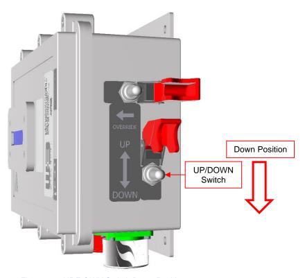
Figure 3-3 UP/DOWN Switch Down Position
