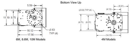
Figure 2-1 Mast Installation Dimensions (Not to Scale)
