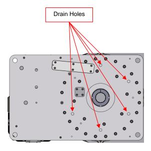
Figure 2-4 Drain Hole Locations
