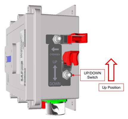
Figure 3-1 UP/DOWN Switch Up Position
