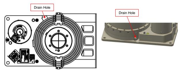
Figure 2-4 Drain Hole Location
