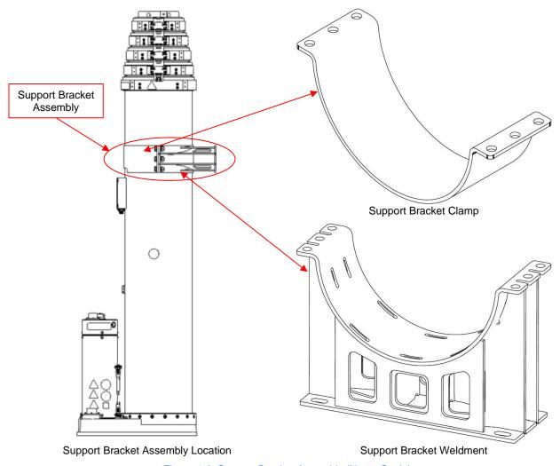
Figure 1-6 Support Bracket Assembly (Not to Scale)
