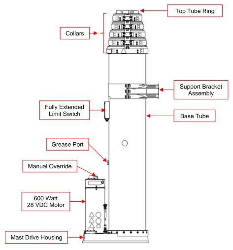
Figure 1-1 Mast (6-Meter Stiletto AL P/N: 711990692 Shown)
