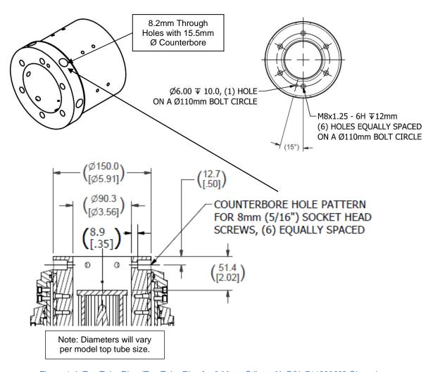
Figure 1-4 Top Tube Ring (Top Tube Ring for 6-Meter Stiletto AL P/N: 711990692 Shown)
