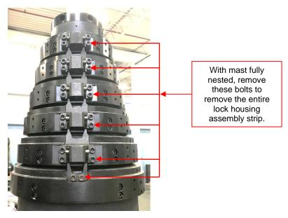
Figure 7 Ensure Mast is Fully Nested
