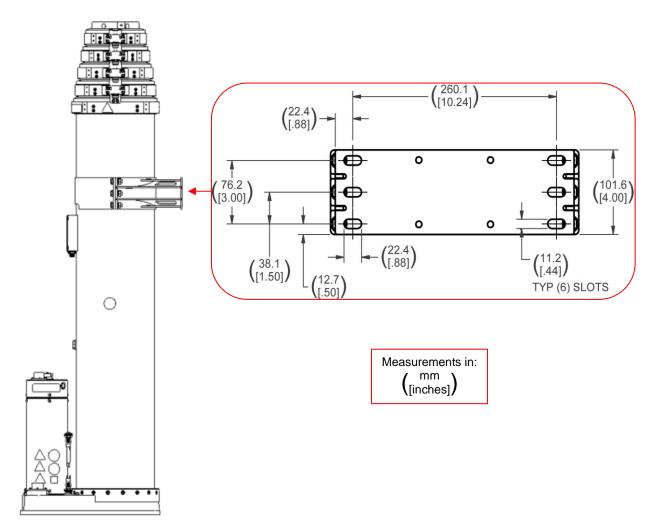
Figure 2-2 Support Bracket Assembly Bolt Hole Pattern
