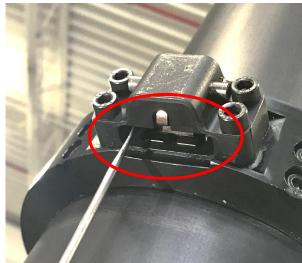
Figure 4 Gently Clean Out Lock Housing Assembly Cavity (Bottom) With Pick
