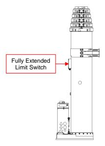
Figure 1-7 Fully Extended Limit Switch
