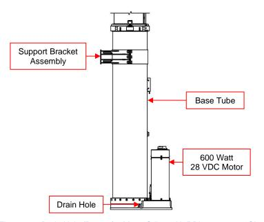
Figure 1-2 Drain Hole (Base of 6-Meter Stiletto AL P/N: 711990692 Shown)
