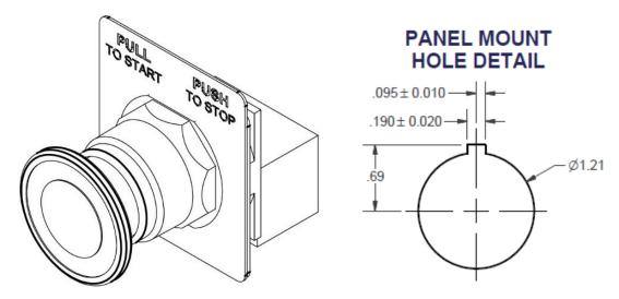
Figure 2-10 Emergency Stop Switch Kit
