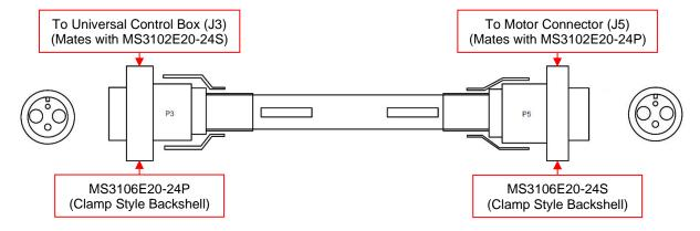
Figure 1-8 Motor and Brake Cable
