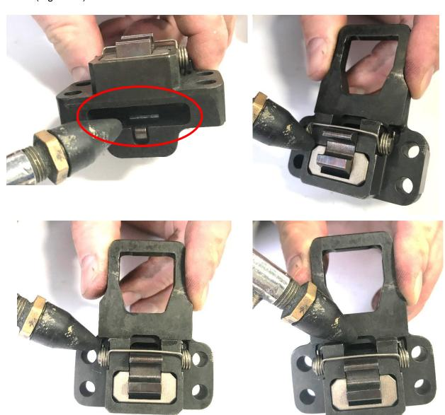
Figure 12 Blow Out Excessive Debris
