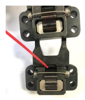
Figure 13 Apply Lubricant in Short, Controlled Bursts
