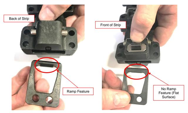
Figure 15 Ramp Feature Must Face the Back of the Lock Housing Assembly Strip
