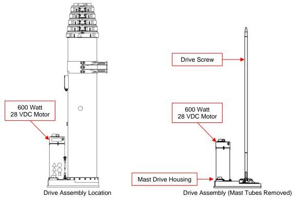
Figure 1-5 Drive Assembly (Not to Scale)
