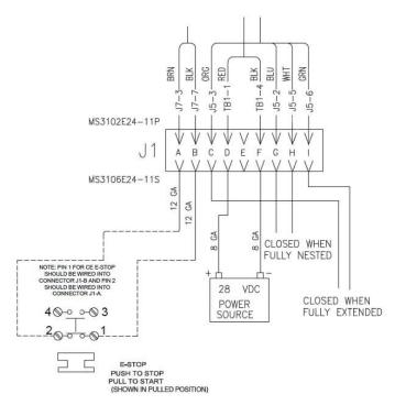
Figure 2-11 Power Cable Connector Wiring
