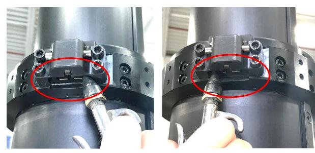
Figure 5 Blow Out Excessive Debris
