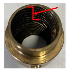
Over 25% Of Threads Worn or Missing
