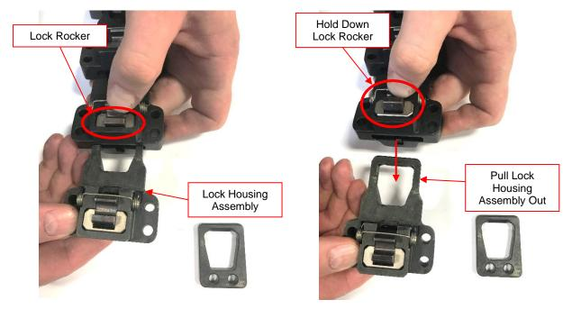
Figure 10 Detach Lock Housing Assembly
