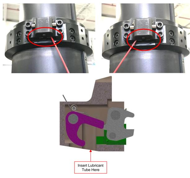
Figure 6 Apply Lubricant in Short, Controlled Bursts
