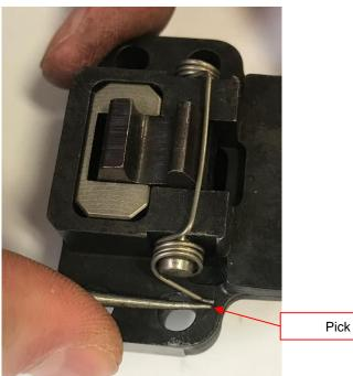
Figure 14 Ensure Corner of Spring is in the Pocket Corner
