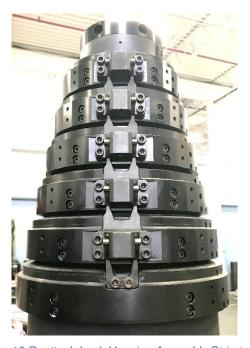
Figure 16 Reattach Lock Housing Assembly Strip to Mast
