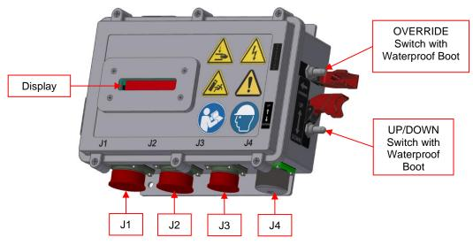
Figure 1-17 Universal Control Box Components
