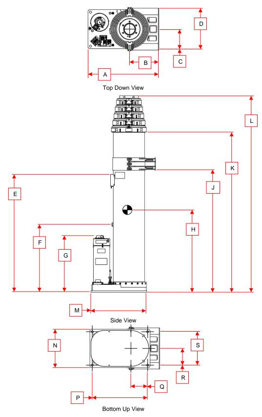
Figure 2-1 Mast Installation Dimensions (Not to Scale)
