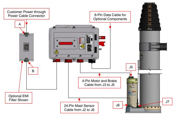
Figure 2-8 Stiletto AL Wiring (Not to Scale)
