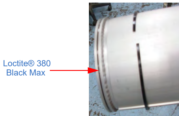
Figure 8-13 Loctite® 380 Black Max in Groove
