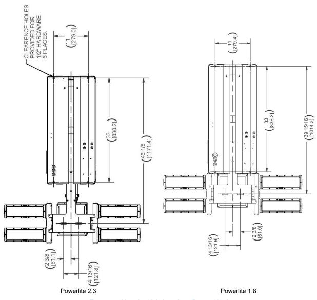
Figure 2-3 Mounting Hole Locations (Bottom View)
