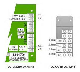
Figure 2-8 Light Power Inputs
