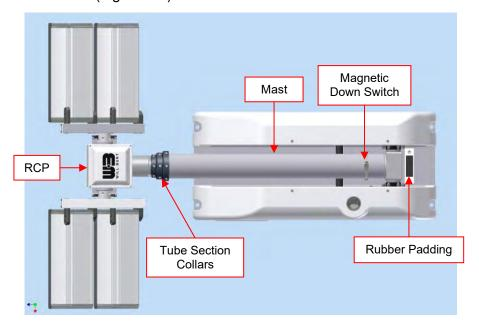
Figure 1-3 Mast Components (Night Scan Chief shown)
