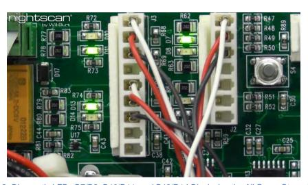
Figure 4-2 Diagnostic LEDs D7/D8, D10/D11, and D13/D14 Displaying the All Green Stowed Position
