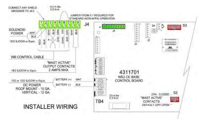
Figure 2-6 Wiring J4
