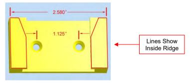
Figure 2-5 Holder for the Controller
