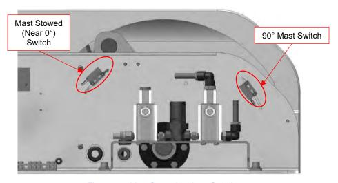
Figure 4-3 Mast Stowed and 90° Switch
