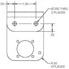
Figure 2-4 Bulkhead Dimensions
