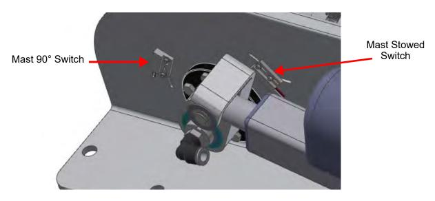
Figure 7-3 Mast Stowed and Mast 90° Limit Switch Locations (Cover Removed)
