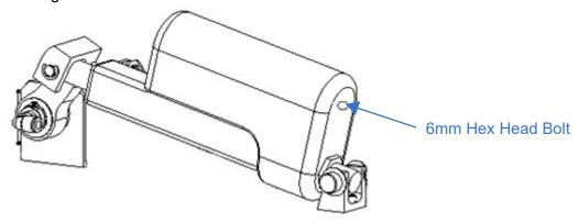
Figure 6-1 Actuator Override for Manual Retraction
