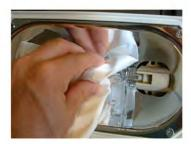
3. Obtain a napkin or towel free from debris, dirt, oil, etc. to remove the lamp.
