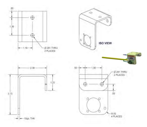
Figure 5-4 HHRC Bulkhead Bracket Installation Dimensions
