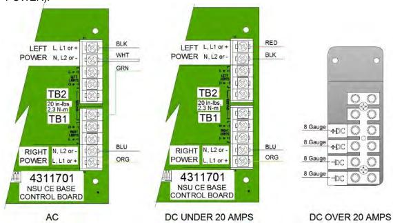
Figure 5-8 Light Power Inputs
