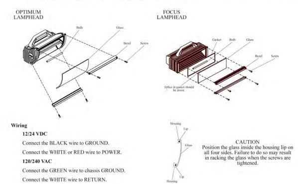
**Bulb Replacement Optimum and Focus Lampheads**
