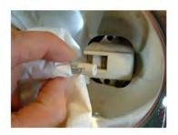
5. Right side of lamp will free if the left, spring-loaded side is pushed all the way in. This may require strong force as the lamp holders are tight.
