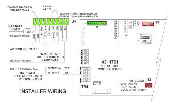
Figure 5-7 Wiring J4
