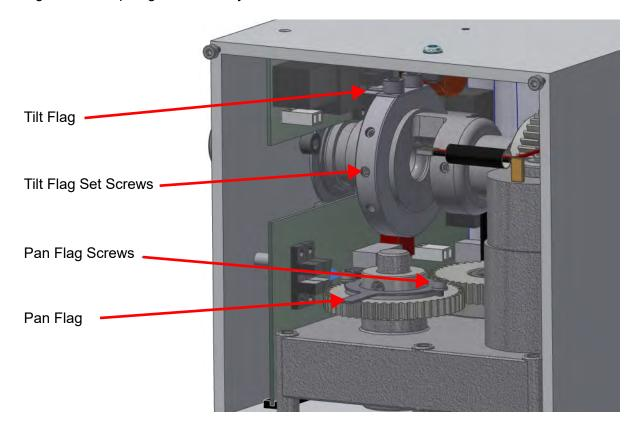
Figure 7-4 RCP Flags (RCP cover removed)
