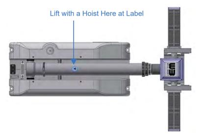
Figure 5-2 Center of Gravity Hoisting Position
