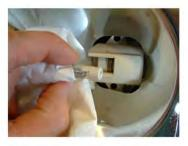
5. Right side of lamp will free if the left, spring-loaded side is pushed all the way in. This may require strong force as the lamp holders are tight.
