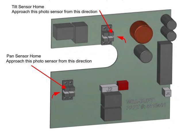
Figure 7-5 RCP PCB Photo Sensors
