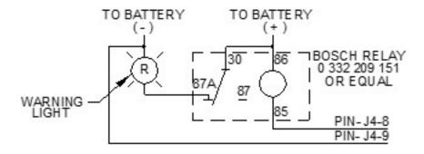
Figure 5-10 Example Vehicle Safety Interconnect Circuit
