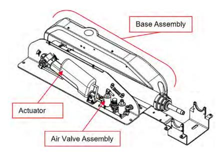
Figure 10-2 Night Scan Chief Base with Air Valve Assembly
