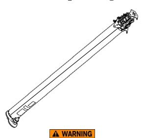
Do not deploy the mast if power lines are less than 80 ft. (24.4 m) from the center of the deployment site.
