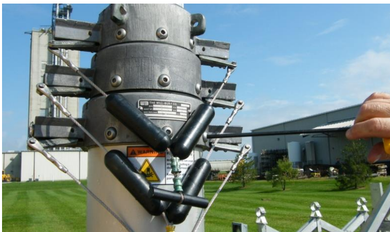
Figure 2-1 Remove One Collar Bolt and Washer from Bottom Section Collar
