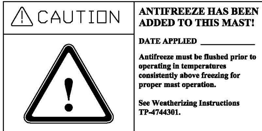
Figure 3-2 Flush Caution Label (P/N: 4770001)
