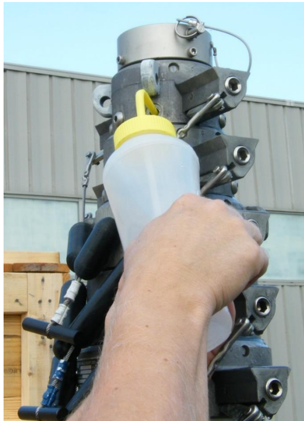
Figure 2-8 Add 32 Ounces of Water to Each Collar
