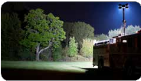
Extends 2 meters above the emergency service vehicle
