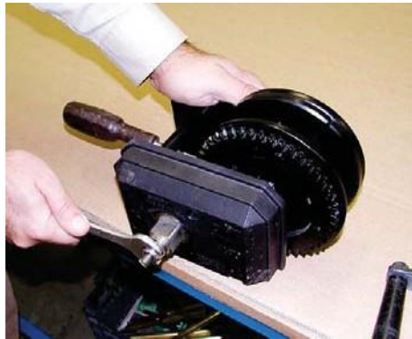
Figure 3-24 Use Wrench to Turn Safety Nut
