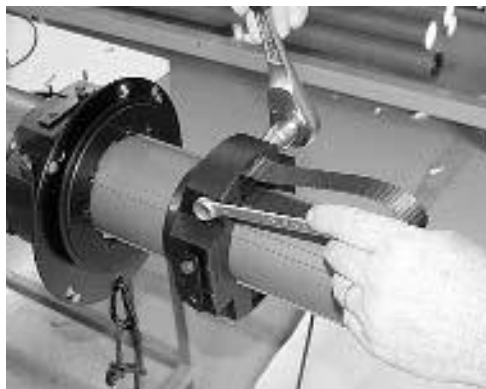
Figure 3-18 Unscrew Running Wheel Axis
