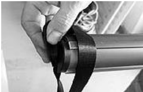
Figure 3-16 Remove Lifting Belt
