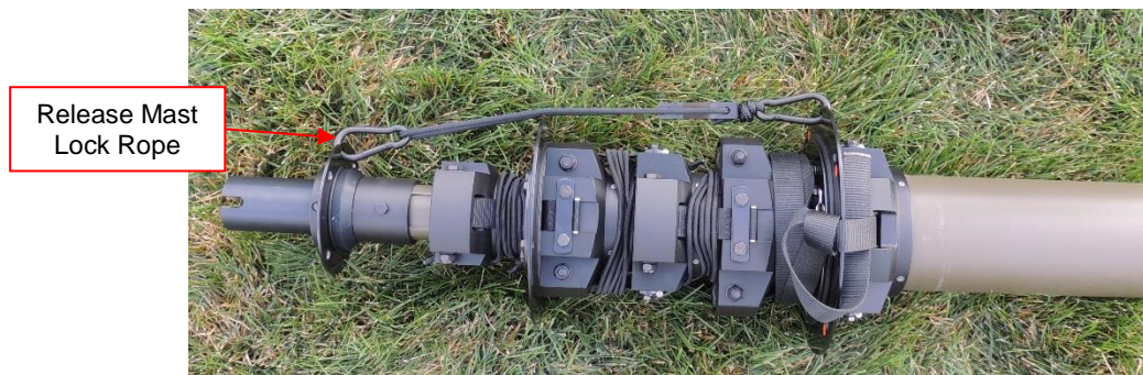
Figure 2-9 Release the Mast Lock Rope
