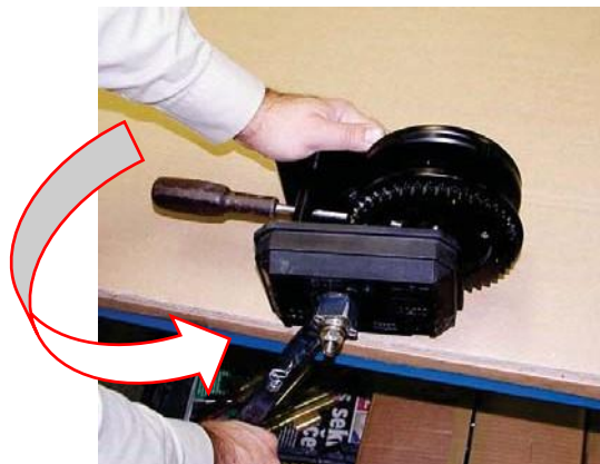
Figure 3-22 Move Crank Counter-Clockwise
