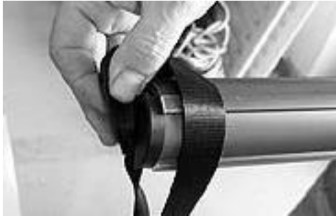
Figure 3-5 Remove Lifting Belt
