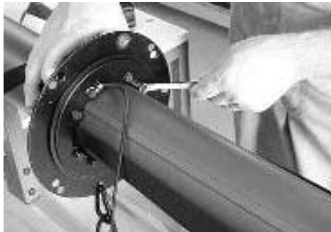
Figure 3-9 Unscrew the Upper Glider
