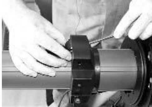
Figure 3-19 Remove the Running Wheel
