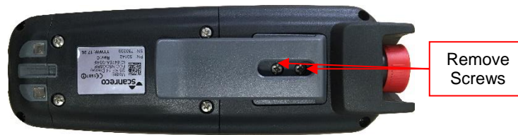
Figure 4-6 Remove Screws Securing Belt Clip
