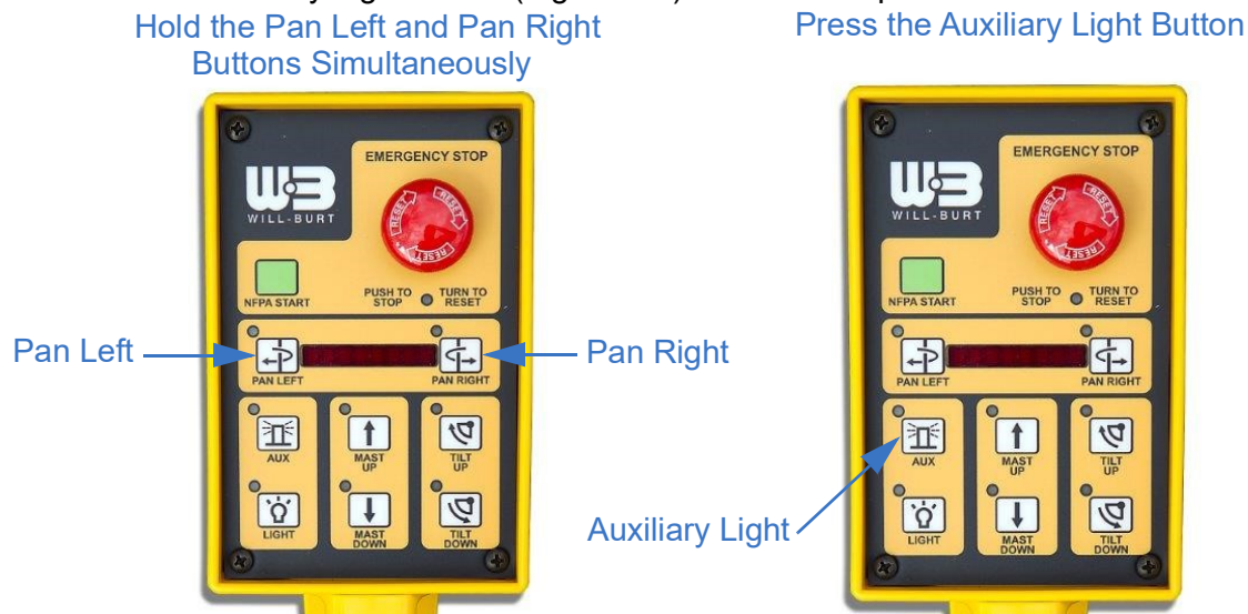
Figure 6-1 Setting the Preset Stowed Position
