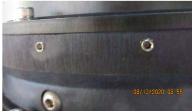
Figure 8-8 Set Screws Flush with Collar Surface
