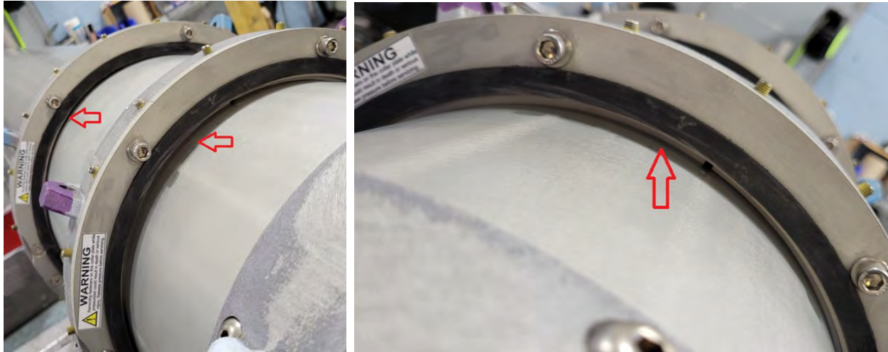
Figure 8-6 Ensure Collars Consistently Center the Intermediate Tube
