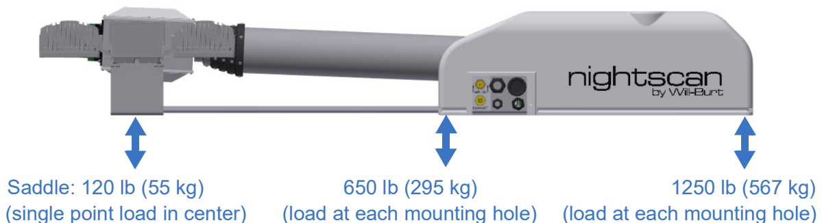
Figure 5-1 Reaction Loads on Mounting Structure
